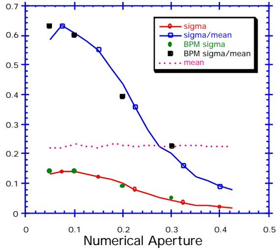
Figure 8. The variation of modal noise with numerical aperture. Standard deviation  $\sigma$  of coupled power is plotted for phase space method (empty markers) and using a finite-difference BPM (filled markers).
